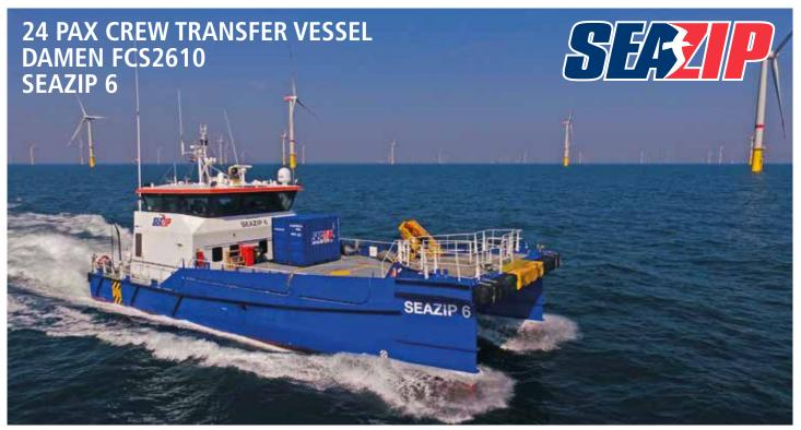
M.V. SeaZip 6 is a fast Twin Axe Bow catamaran for transport of personnel, equipment and parts to offshore windfarms, etc.
